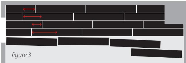
5. The first row: Starting in the corner, working from left to right, install the first full row of tiles/planks along the chalk line. It is critical that the first row be straight as it is the foundation for the rest of the installation.
